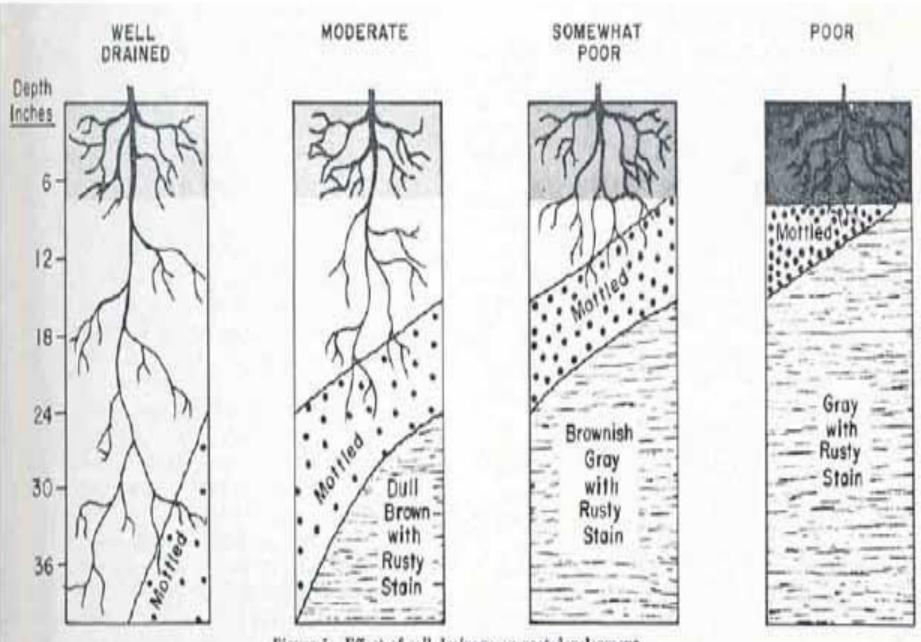
Figure 5.-Effect of soil drainage on root development.
